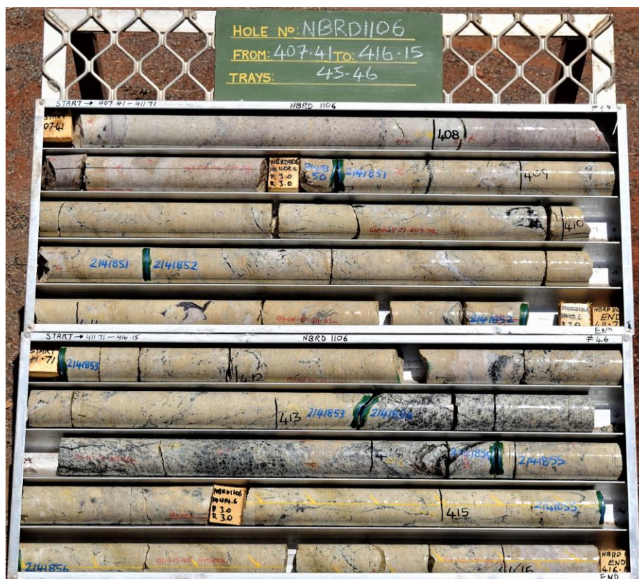
Figure 2: Apatite-rich mineralization intersected in deep exploration hole NBRD1106 (North Zone). This 8.74 m interval contains about 6% TREO, 25% P 2 O 5 and has an NdPr Enrichment of 27.0%.
