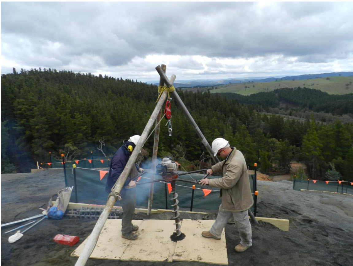
Figure 4-1 Power auger sampling of Lloyds Mine tailings.
