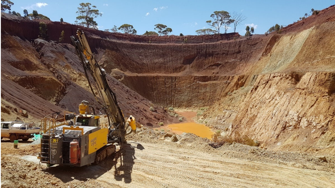
Figure 2 – RC Drilling at Panther Prospect
