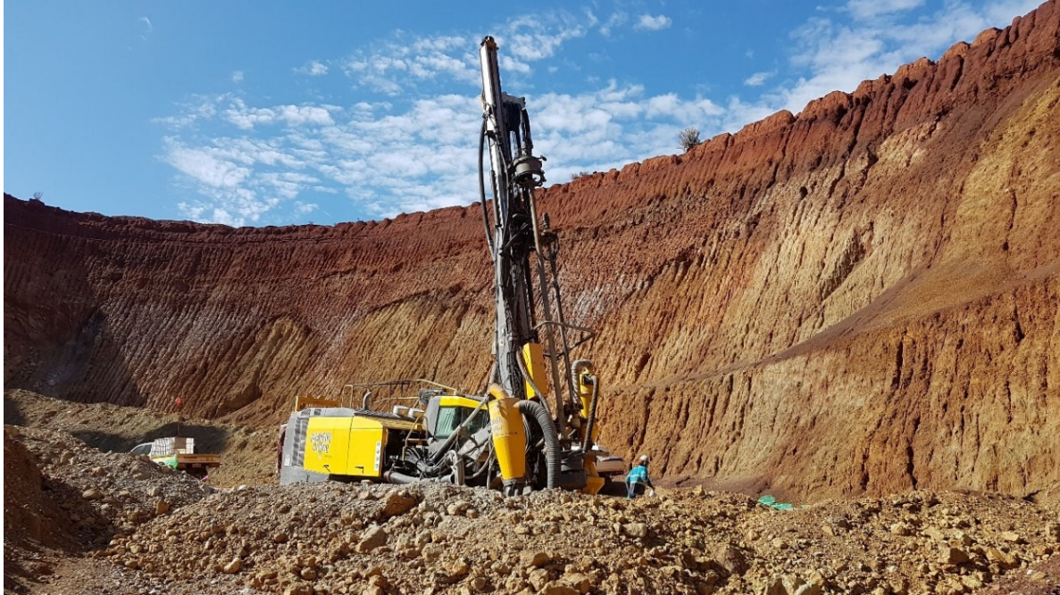
Figure 8: Second phase of RC drilling at the Panther deposit
