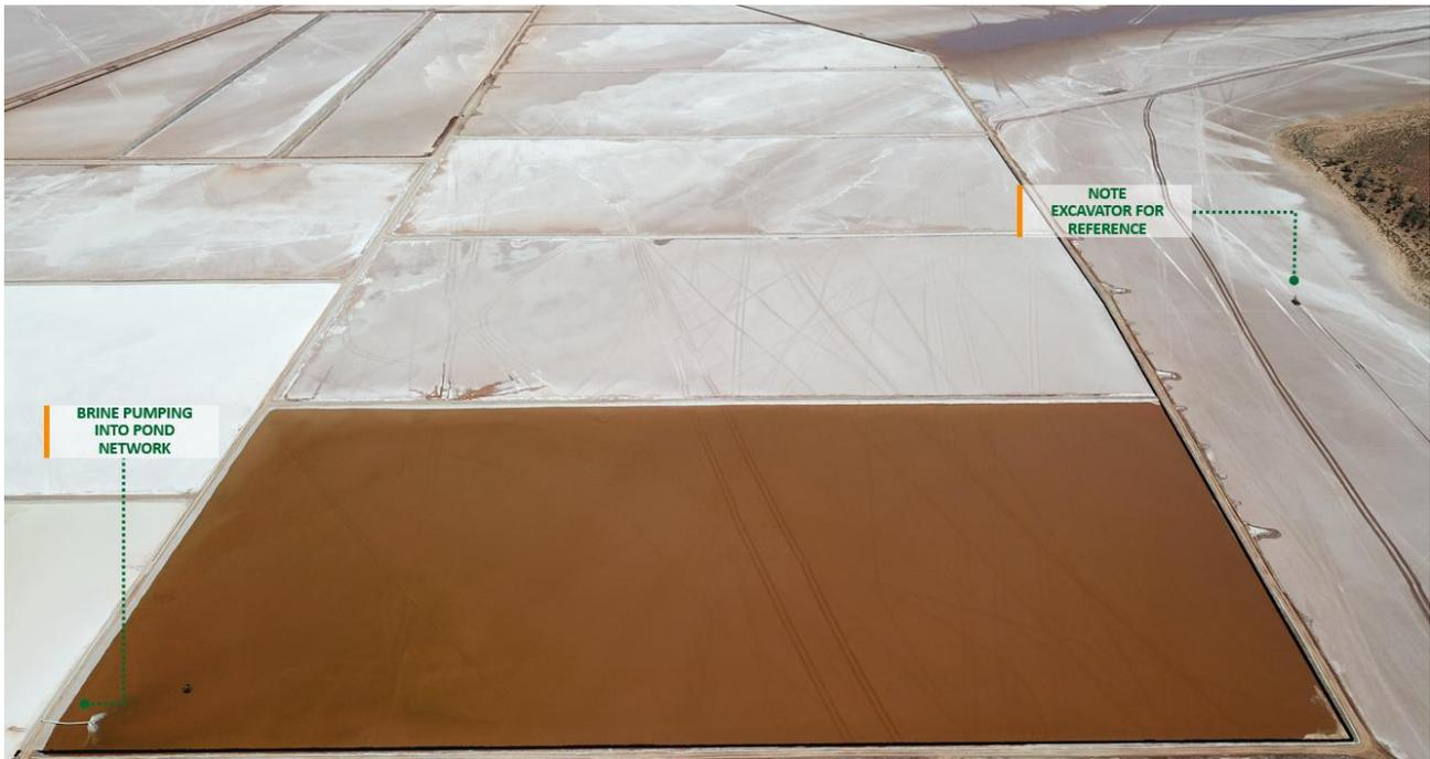
Figure 1: Stage 2 Pond network filling with brine
