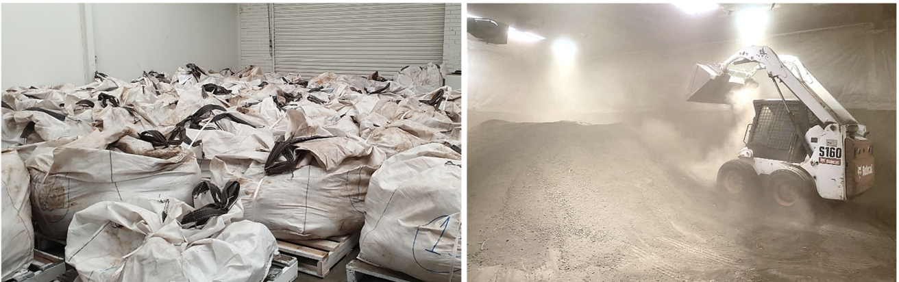
Figure 8 and 9 : Part of the 60 tonnes bulk sample at ALS laboratories in Perth, right: in bulka bags on arrival; left: being mixed and combined to produce a homogenised feed for the pilot plant
