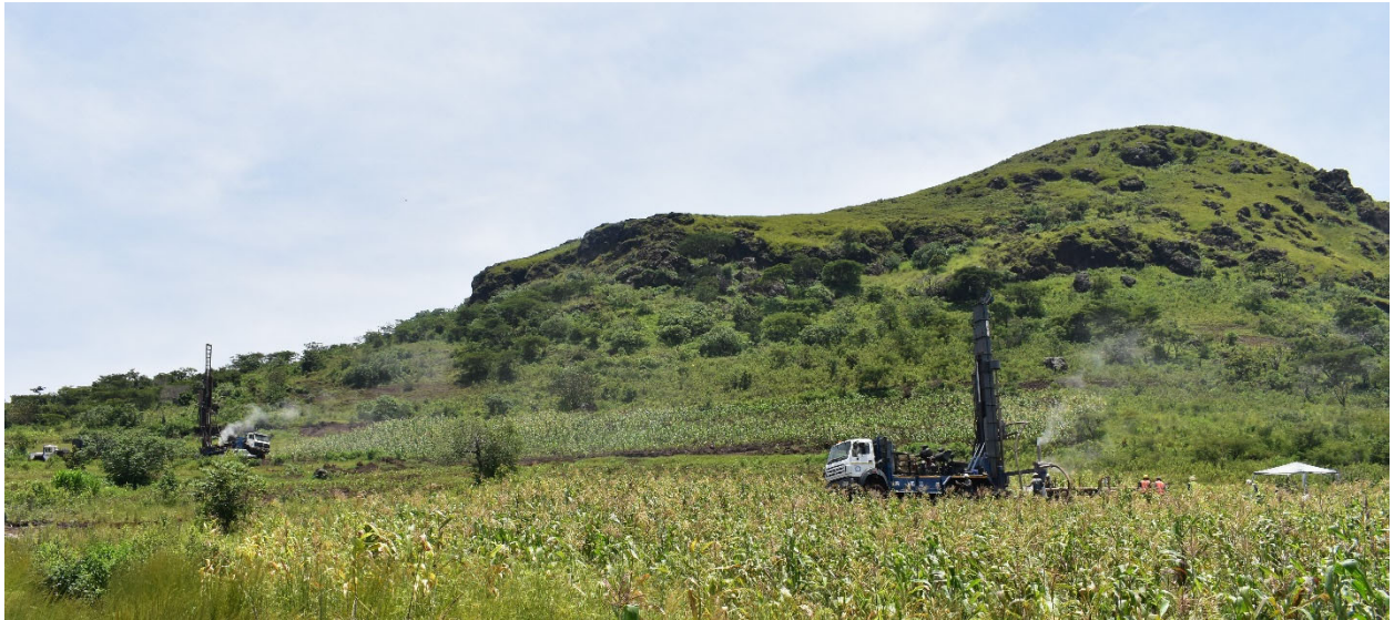
Figure 2: Two reverse circulation drill rigs in operation in the main mineralised zone at Longonjo, February 2020.
