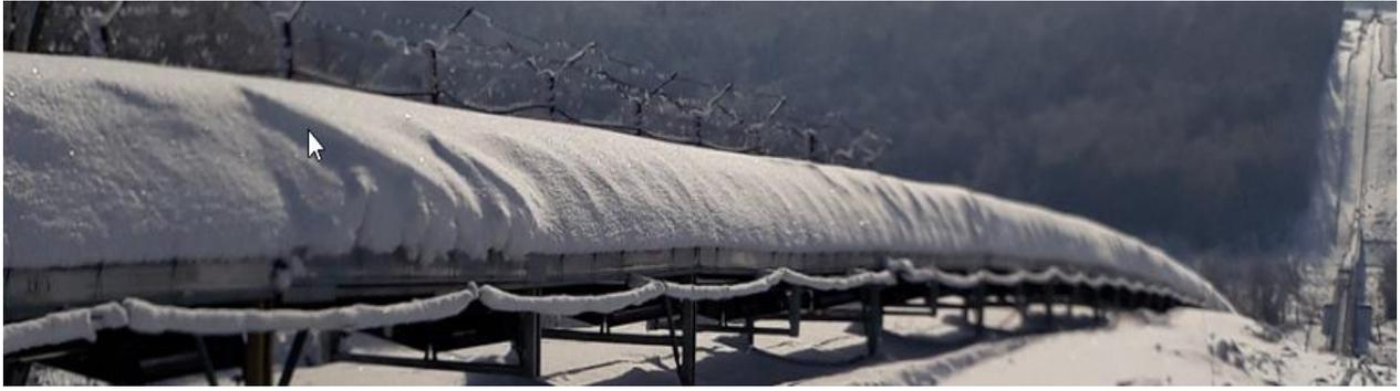
**Figure 10: Example of covered overland conveyor system**
