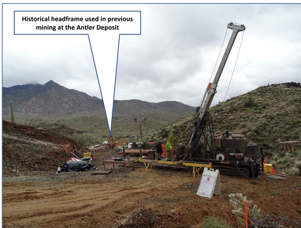
Diamond core drilling rig in operation at the Antler Copper Deposit.
