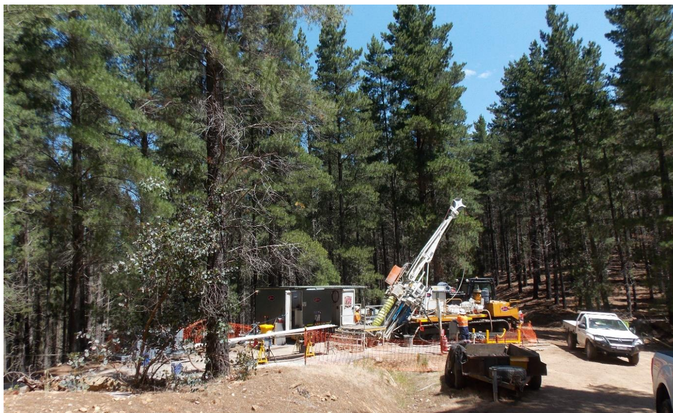
Photo of Deepcore Drilling LF30 diamond drill rig set-up on hole MU19DD01 of the Mustang Prospect (Nov 2019). Note that the rig is set-up on an existing track without the need for any ground disturbance.
