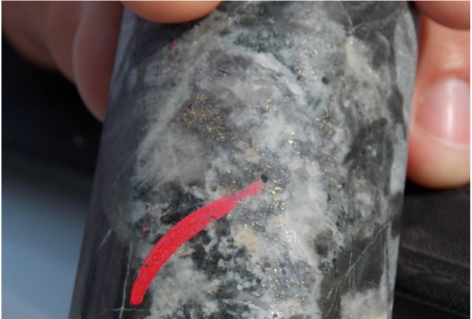
ASX: KZR 23 December 2019: Photo of fine grained (sub-mm) disseminated visible gold and associated arsenopyrite intersected in MU19DD04 from 100.32m. Length of core shown is approximately 6cm.
