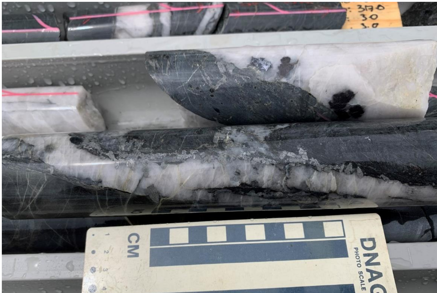
ASX: KZR 23 December 2019: Mineralised quartz veins and sulphide alteration assemblages observed in MU19DD02 (approx. 319.6m). Note coarse grained euhedral arsenopyrite grains (foreground core sample), coarse-grained galena and sphalerite (background core sample) found near margins of quartz vein.
