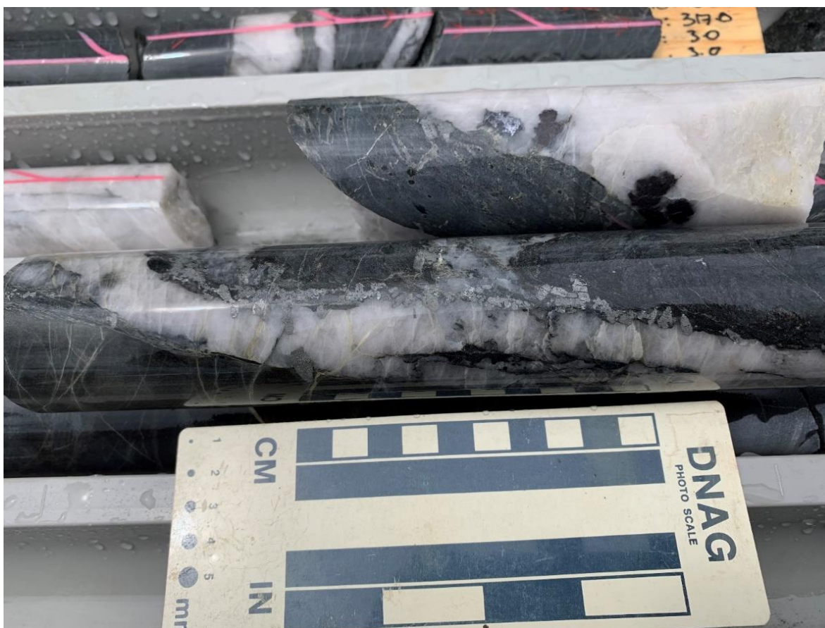
Figure 2: Close up photograph of mineralised quartz veins and sulphide alteration assemblages observed in MU19DD02 (at approximately 319.6m). Note coarse grained euhedral arsenopyrite grains (foreground core sample) and coarse grained galena and sphalerite (background core sample) found near the margins of the quartz vein.
