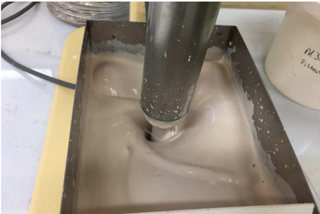
Attrition test at 30% density (70% water), providing optimal results for high Al 2 O 3 grade and recovery at 10 & 7.5 minutes
