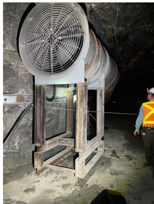
Photo 8 – Underground Secondary Fan
