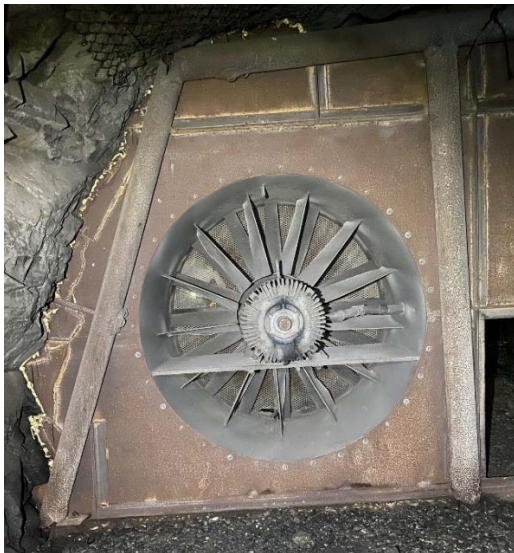
Photo 5 – Underground Ventilation Fan
