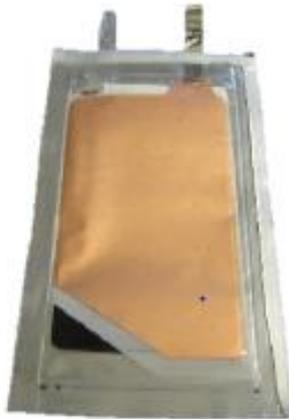
**Image 1: Image of a single-layer pouch test cell**
