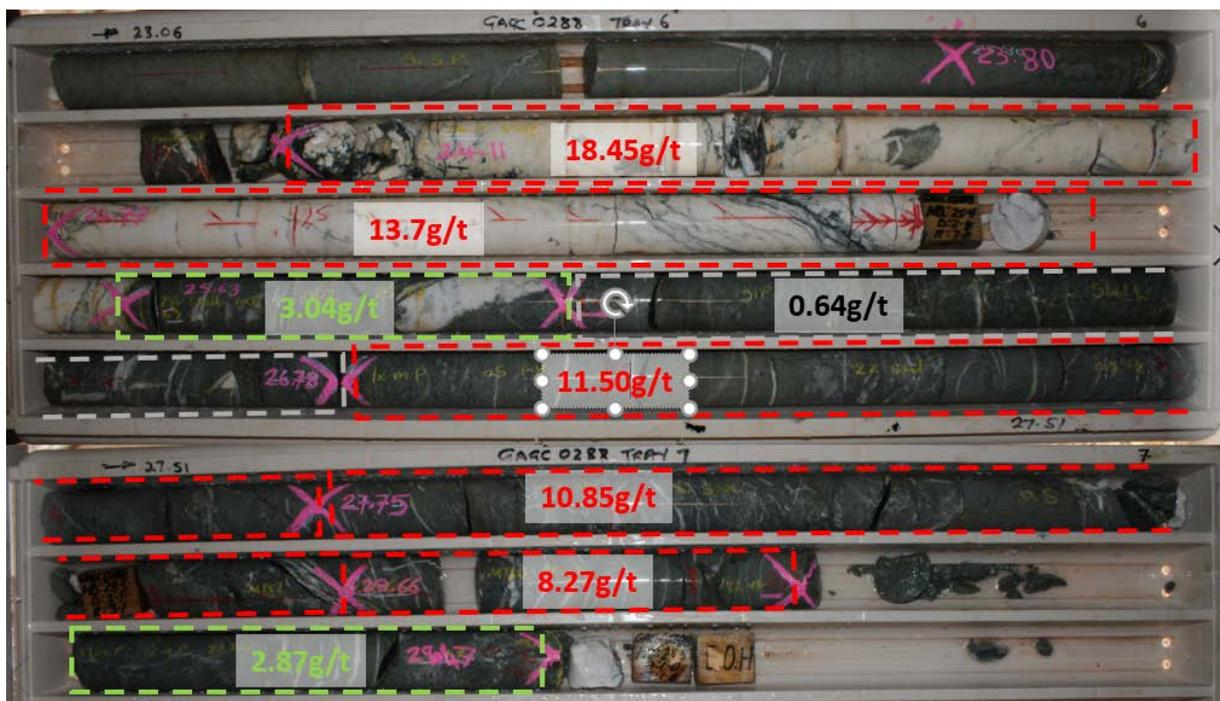
Figure 2: GAGC0288 drill core with assays and high-grade quartz reef mineralisation.
