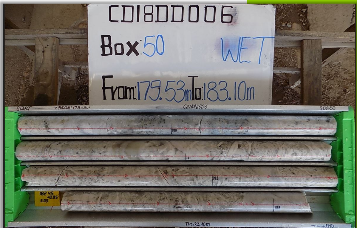
Figure 4: CD18DD006. 181 – 182m 4.65% contained \text{Li}_2\text{O}
