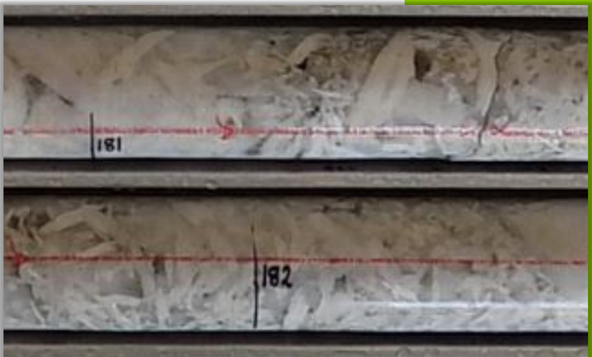
Figure 5: Close up of core from 181 to 182 metres. Very coarse spodumene throughout photo is out of focus
