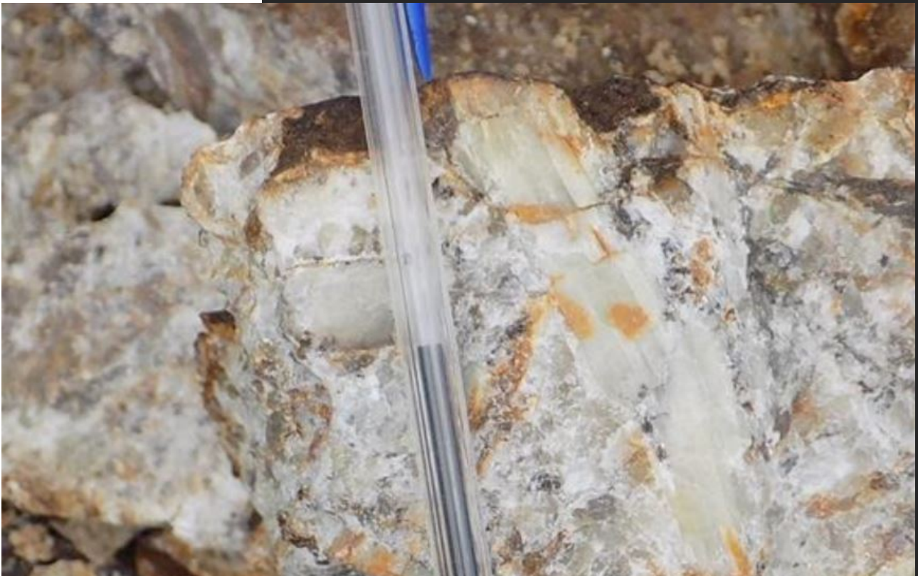
Figure 5: Rock Chip Sample collected showing white spodumene (the large, long prism to right of the blue pen) in a quartz feldspar matrix
