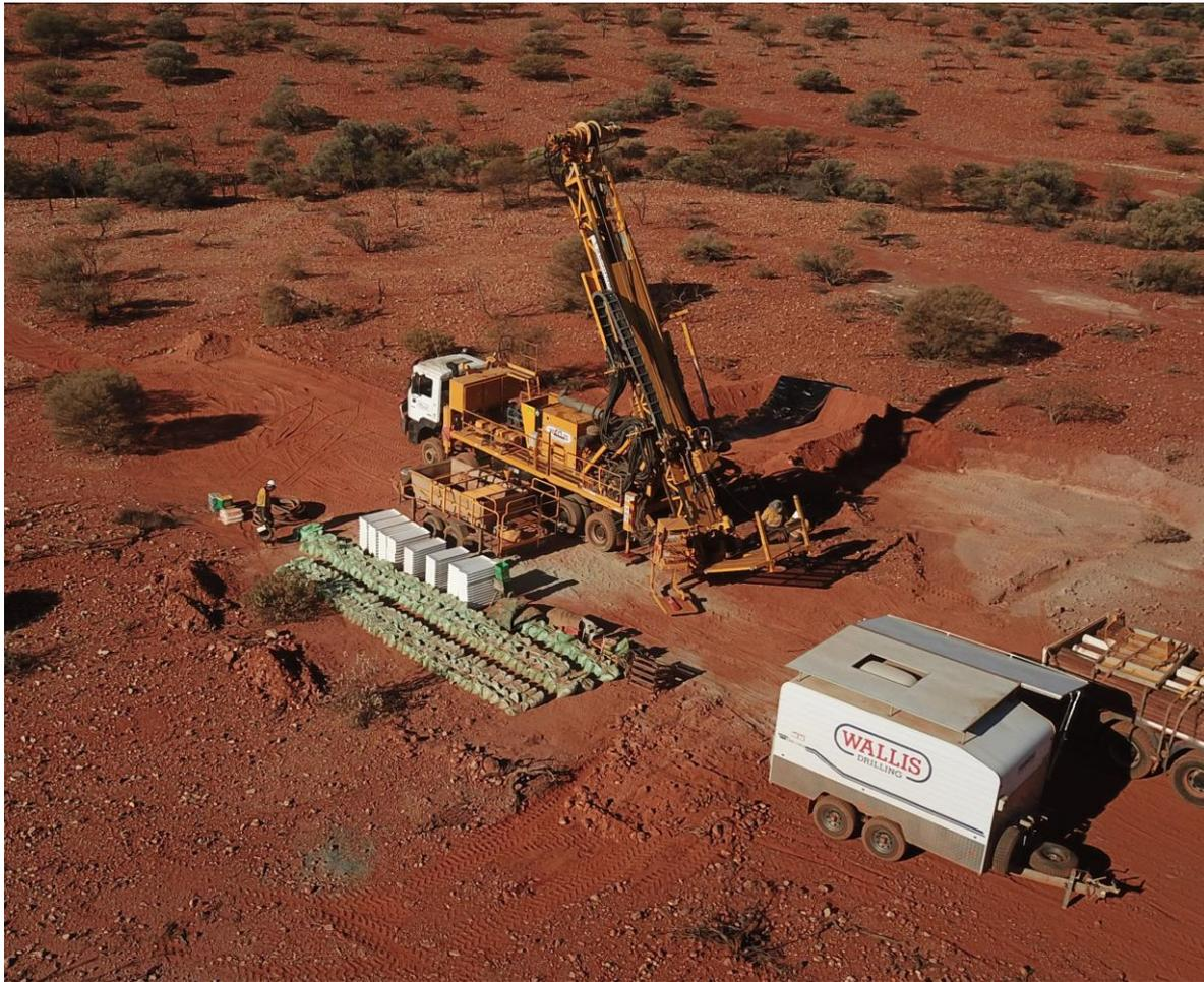
Figure 1: Diamond drilling at Kingsley commencing
