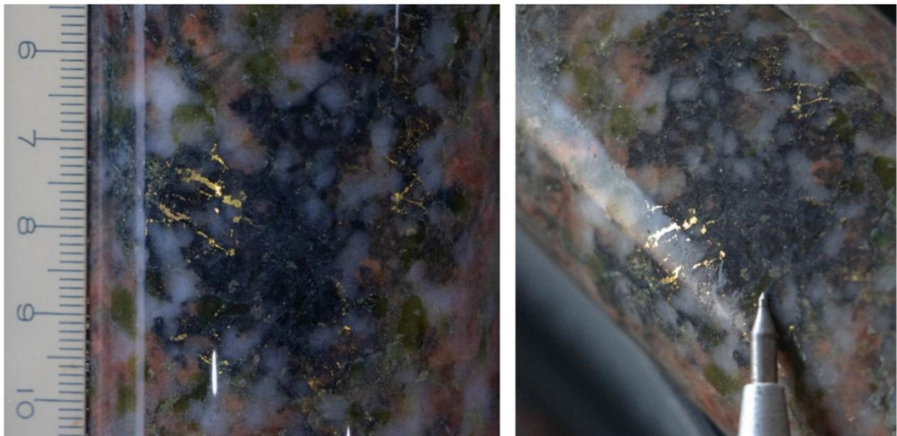
**Figure 3:** Free gold within intensely sericite +pyrite +phengite + chlorite + quartz altered granite from DDH JUDD001
