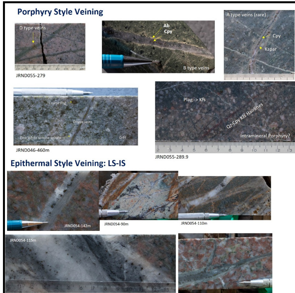
Figure IX. Juruena drill cores exhibiting porphyry style and epithermal veins frequently associated with Au-Cu mineralisation.
