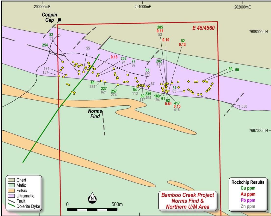
Figure 5: Map of the Northern Prospect Area and the 100 new sample results in this area
