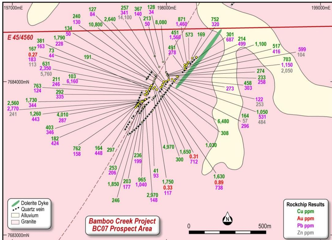
Figure 8: View of the BC07 Prospect Area (E45/4560) and All rock sample results to date
