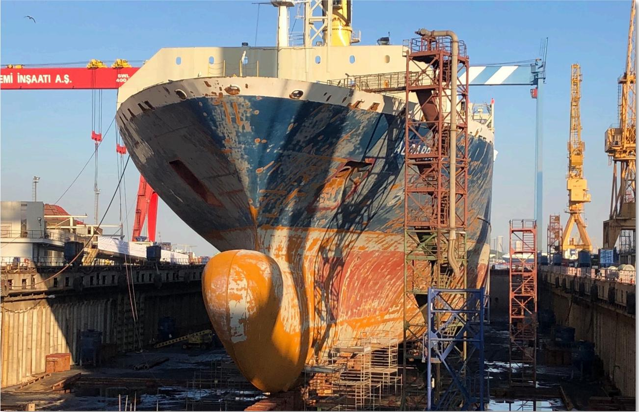
**Figure 3** Talphene®-enhanced primer (left) being spray coated onto starboard hull of vessel, alongside the test reference coating (right).
