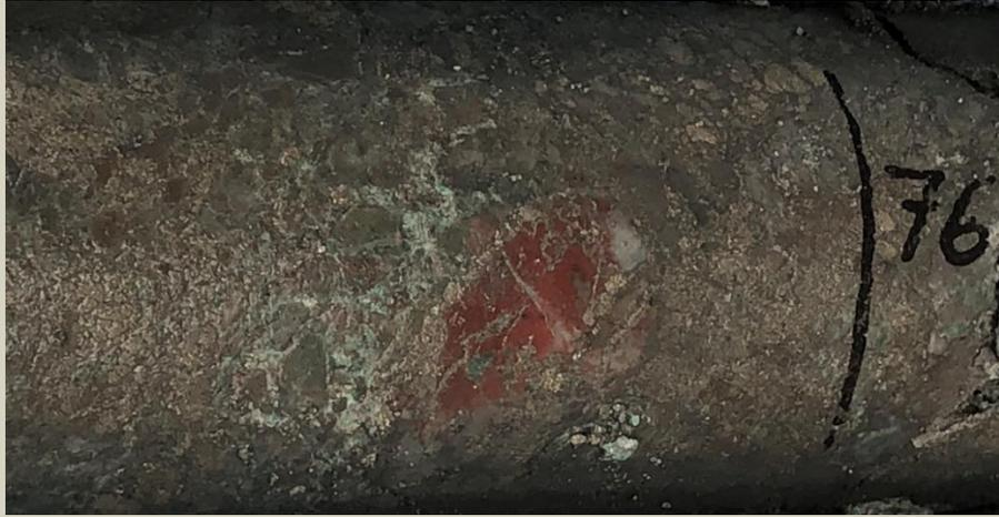
Structural / hydrothermal breccia with quartz-hematite altered siltstone clast and semi-massive sulphide, pyrite-clay matrix. 75.9m.
