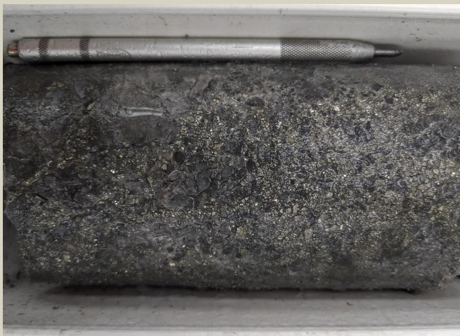
Semi-massive sulphide in a sandstone protolith at 43.4m.
