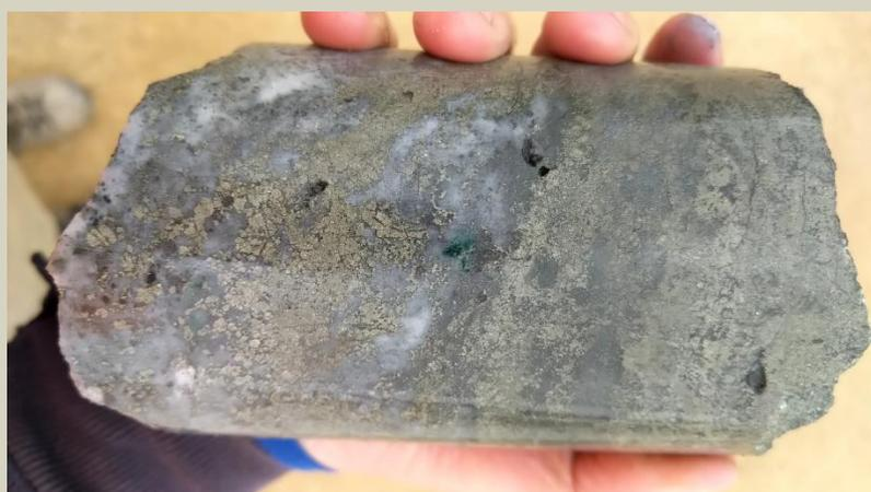
Massive pyrite with silica alteration and chalcopyrite at 92.6m.
