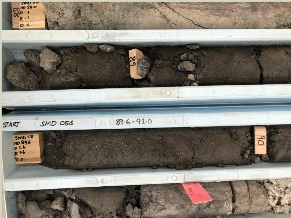
Massive sulphide lens comprising 85-90% pyrite, 10-15% sooty black chalcocite and 1-2% chalcopyrite. 88.4-91.2m.
