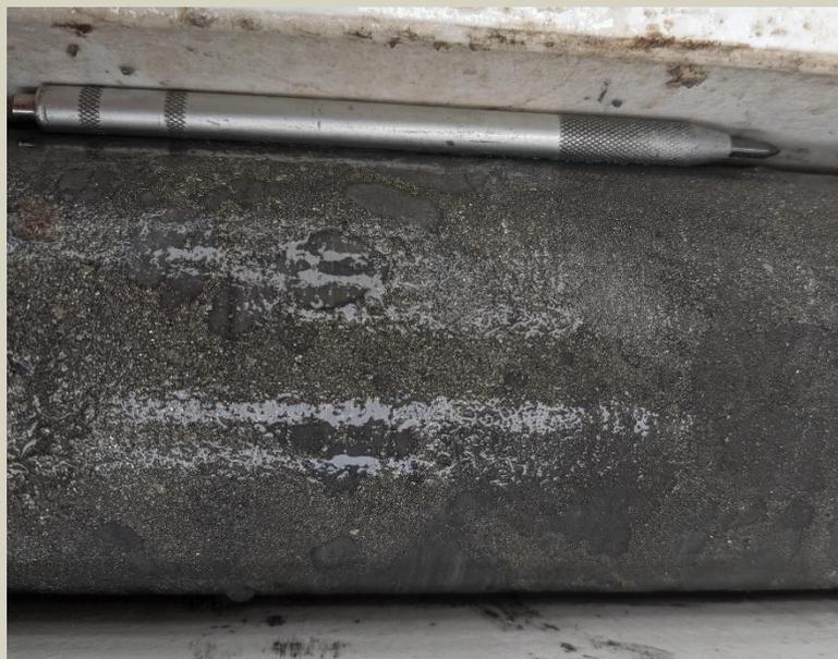
Massive pyrite sulphide zone at 53.9m.
