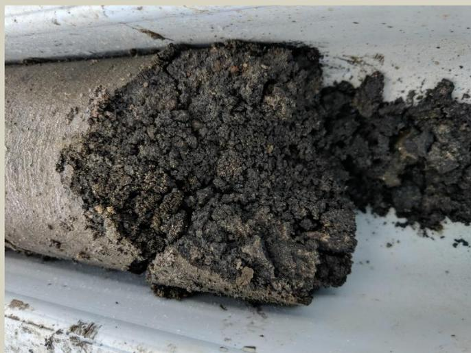
Massive chalcocite mineralisation at 94.4m.
