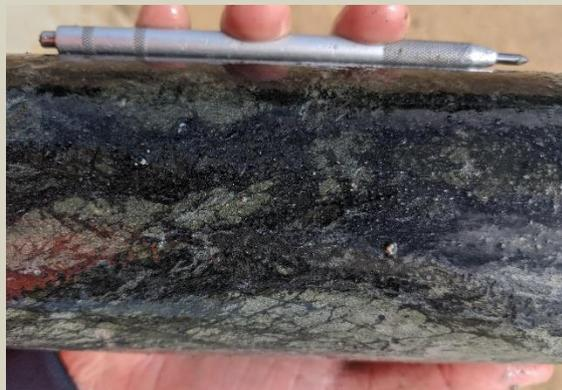
Serpentinite with strong magnetite alteration at 111.4m.
