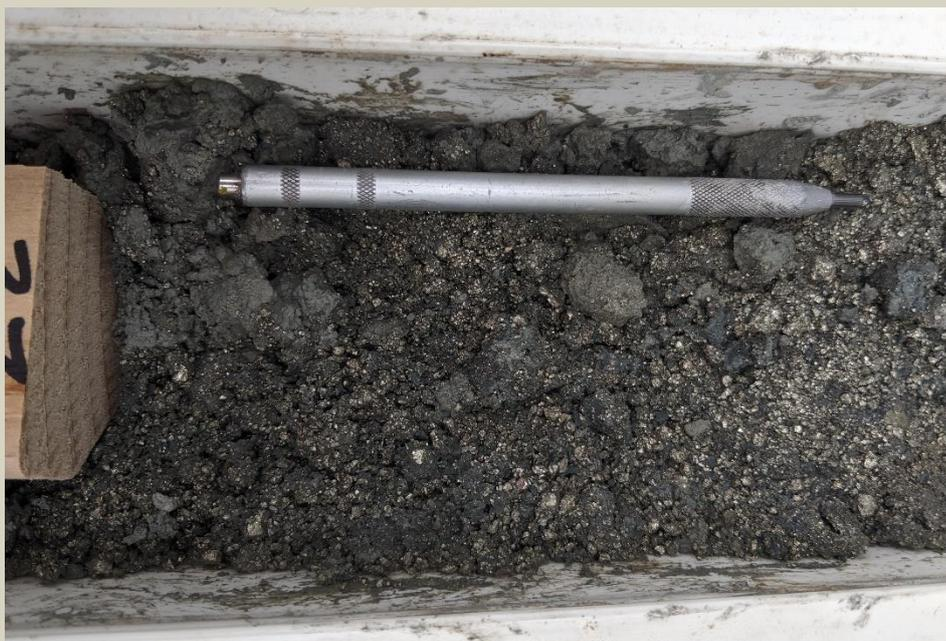
Massive pyrite and trace chalcocite vein at 37.1m.
