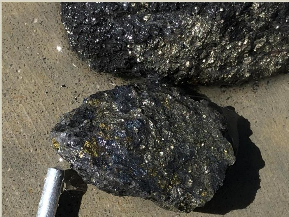
Massive pyrite-chalcocite-chalcopyrite. 89.1m.
