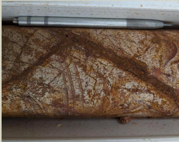
Limonite on fracture surfaces within a sandstone unit at 11.8m.
