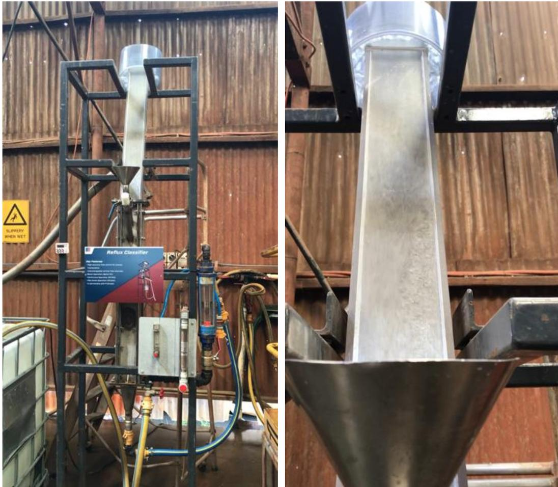
Figure 2: Bench scale Up Current or Reflux Classifier for Mica removal
