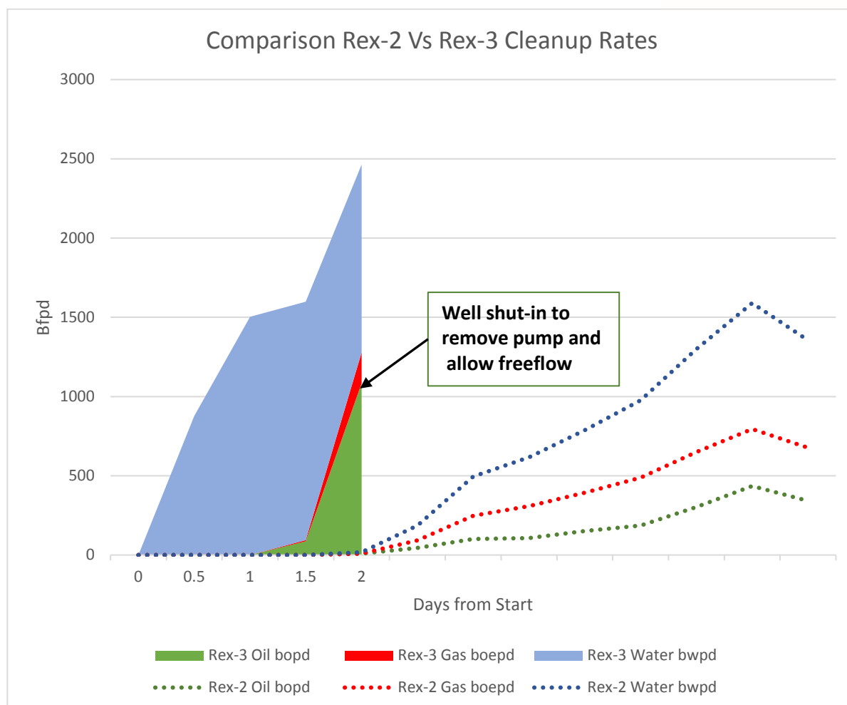
Figure 1 –Comparison of Rex-3 and Rex -2 initial test results
