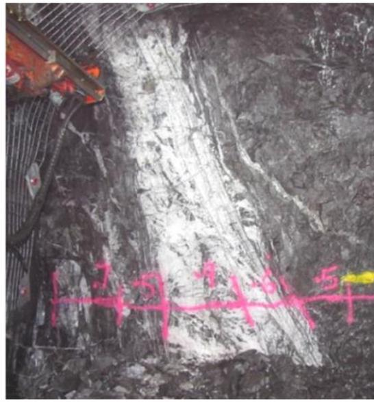
Figure 2: Narrow high-grade vein in development drive at East Kundana. Note the estimated average width of approximately 1.0m.
