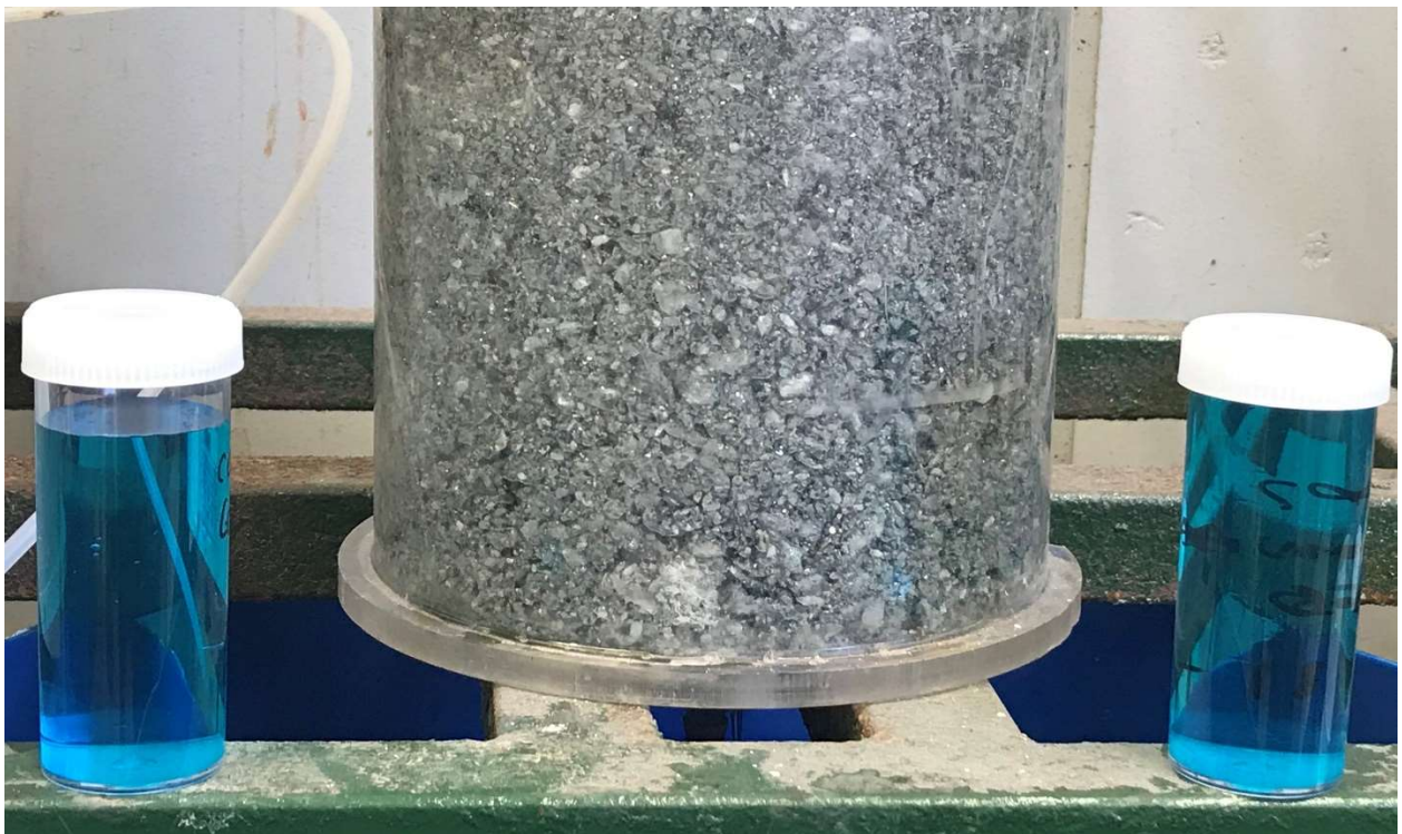
Image 1 / Metallurgical column test-work
