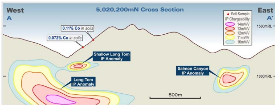
Cross section showing location of, and depths to, some of the chargeability (IP) anomalies at the Colson Cobalt-Copper Project, Idaho.
