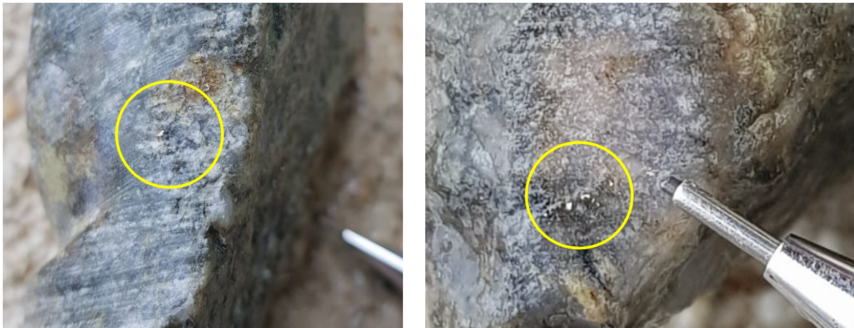
Figure 1. Very fine-grained visible gold in hole NADD001 (118.7 – 120.1) Pencil tip is 0.5mm for scale
