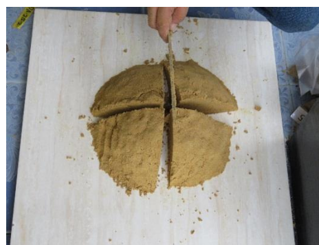
Figure 3-6 Cone and quartering of samples
