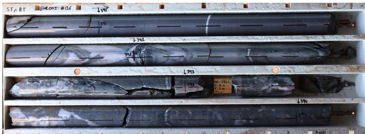
Figure 5 - Quartz and sulphide veining intersected at Anomaly 16 (390.8m-394.1m)
