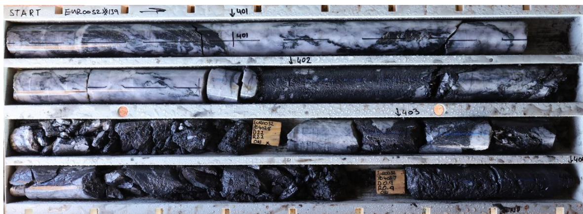
Figure 6 - Quartz and sulphide veining intersected at Anomaly 16 (400.6m-404m)
