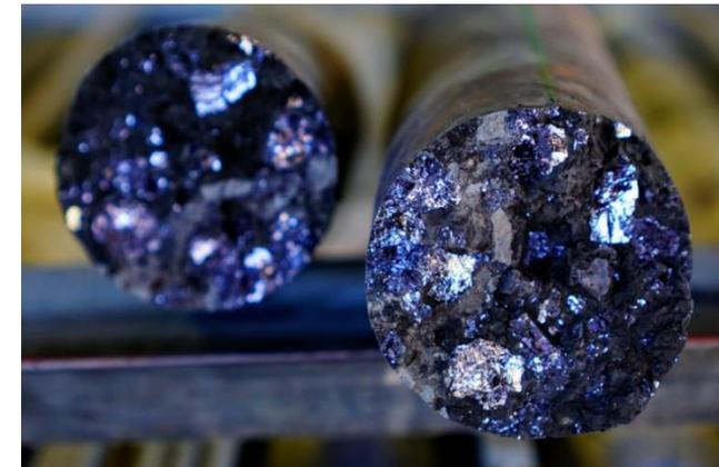
*Image<sup>3</sup>: Crystalline Galena in ACD080 32.8m (Freshly Broken Core). Part of an Interval 25.7m to 37.9m of Well Mineralised Core Consisting of Strong Galena, Some Pyrite and Minor Sphalerite.*
