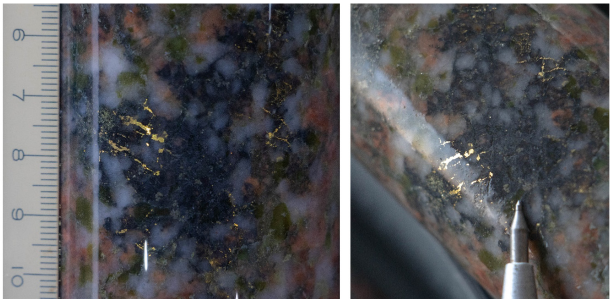
Figure 1: Free gold within intensely sericite, pyrite, chlorite quartz altered granite from DDH JUDD001
