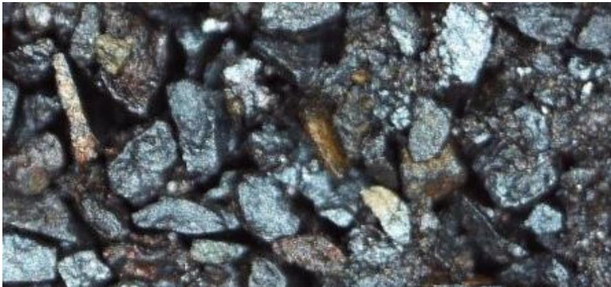
*Figure 1 Magnetic concentrate sample from 6 tonne pilot*
