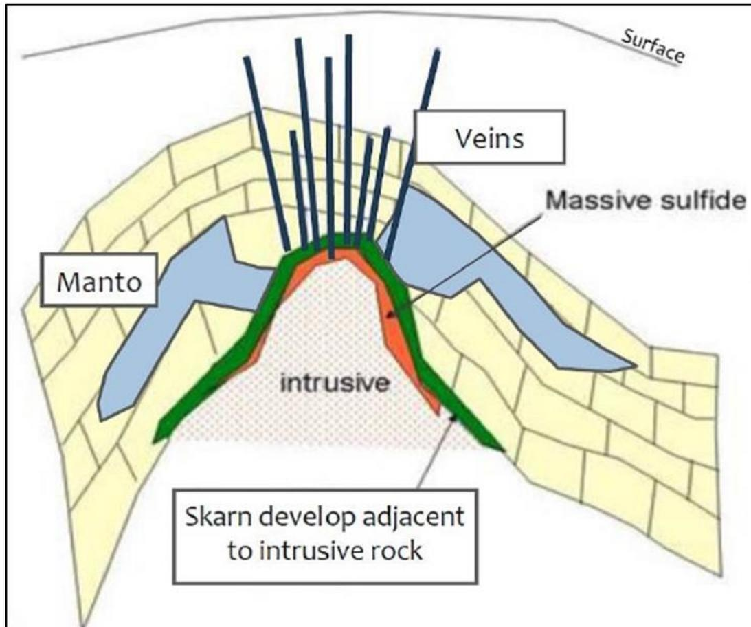
**Figure 1: - Schematic diagram of manto-style mineralisation in carbonate rocks**
