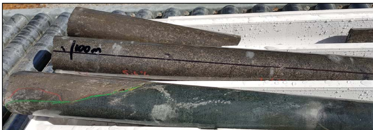
Figure 1 - Photo of diamond core from drill hole EMD002. Massive Nickel Sulphide (grading 6.11% Nickel) is clearly identifiable above a sharp contact with the underlying basalt.
