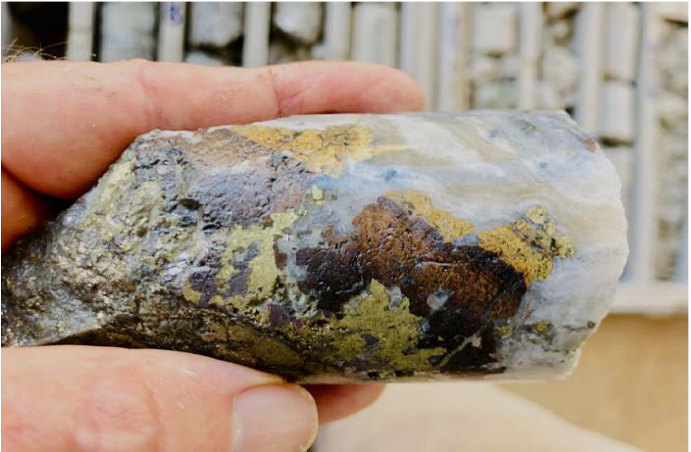
Figure 19. Diamond drill core from 230 metres downhole in RTIPT016. Copper sulphides (chalcopyrite) is yellow coloured at base of core; brown to honey coloured zinc sulphide (sphalerite) in the centre; and colloform to crustiform quartz-chalcedony in upper right.
