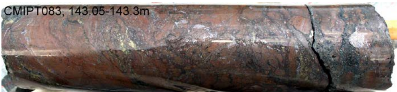
Figure 11. Hole CMIPT083: massive and brecciated massive sphalerite (red-brown) with lesser galena. Up to 3% chalcopyrite (yellow) is present in places.
