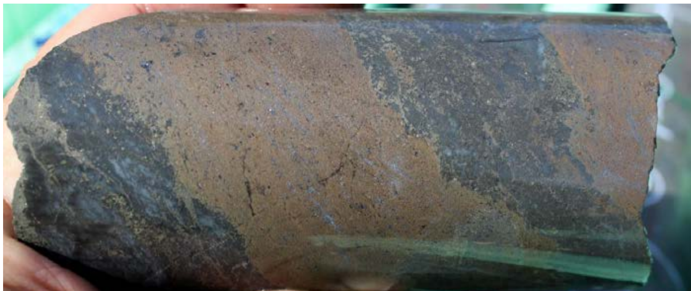
Figure 10. Hole CMIPT084: Photographs of end-member styles of massive sulphide mineralisation: massive pyrite (bronze colour) with fine grained sphalerite and galena (upper) and massive sphalerite (red-brown) with galena (silver grey) (lower). Similar styles of mineralisation occur in all four new drill holes at Main Shaft.
