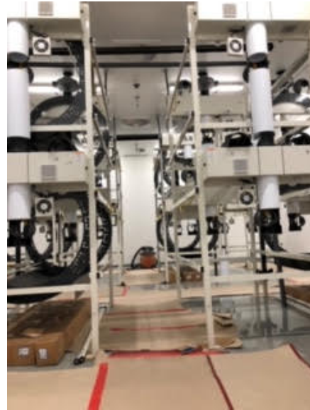
Photo 4: RotoGro Hydroponic Rotational Garden Systems plumbed into ceiling services
