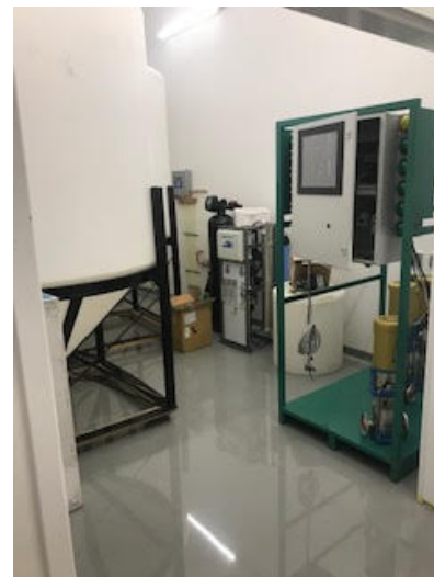
Photo 6: Global Fertigation Solutions Tanks and Fertigation System
