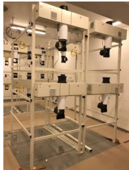
Photo 2: RotoGro Hydroponic Rotational Garden Systems framed in pods of four
