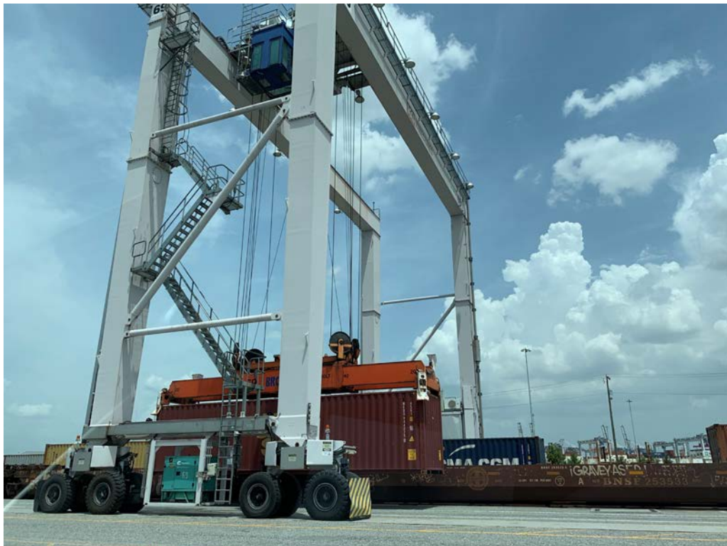
Figure 1. Container crane at Port of Savannah showing wheels on “runway”
