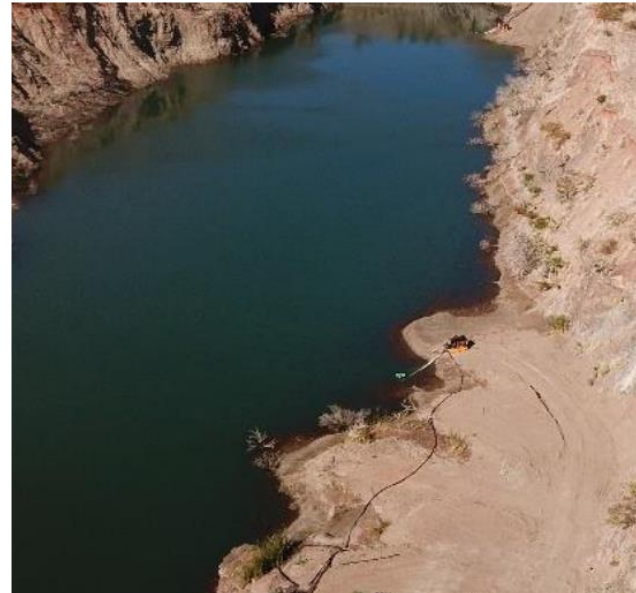
Dewatering underway at the Mt Freda open pit
