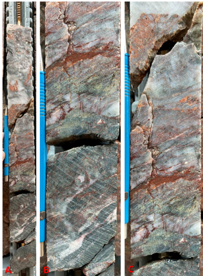
Photo 4: Abundant quartz veins with chlorite, phengite and pyrite (3.4m @ 10.10 g/t Au). (A) General view of the quartz veining; (B) & (C) Detail of the oxidized zones associated with sulphides.
