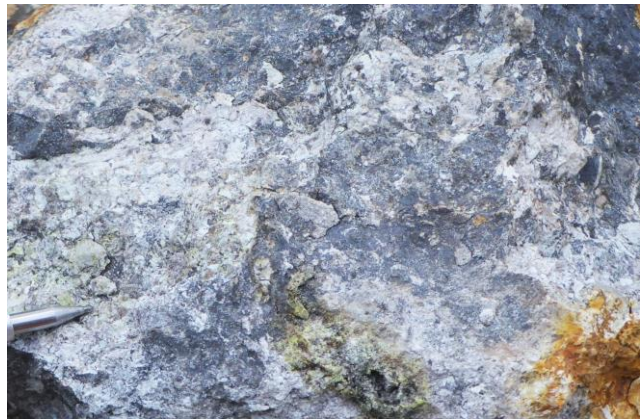
Figure 5 ABOVE LEFT: Sample from an epithermal vein at Colina Roja with 6.5g/t gold and 194g/t silver; ABOVE RIGHT: Sample from an epithermal vein at Uchpanga with 2.65/t gold and 920g/t silver.
