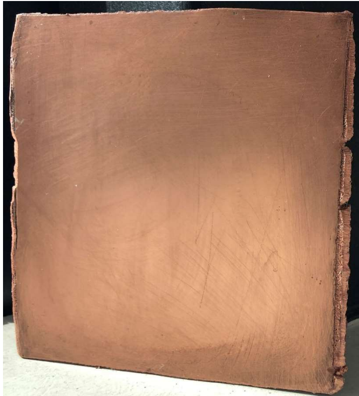
Image 1 / CYM copper plate produced from metallurgical EW test-work
