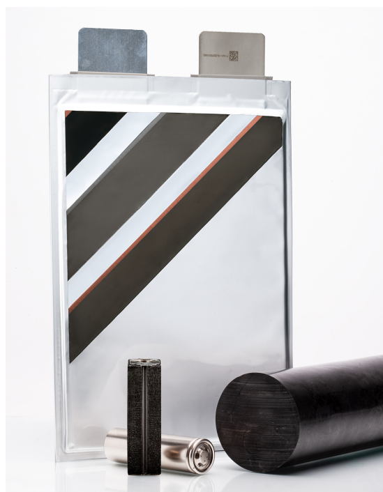
Figure 2. Vittangi graphite ore together with battery pouch cell and cylindrical battery cut to expose the graphite anode.
