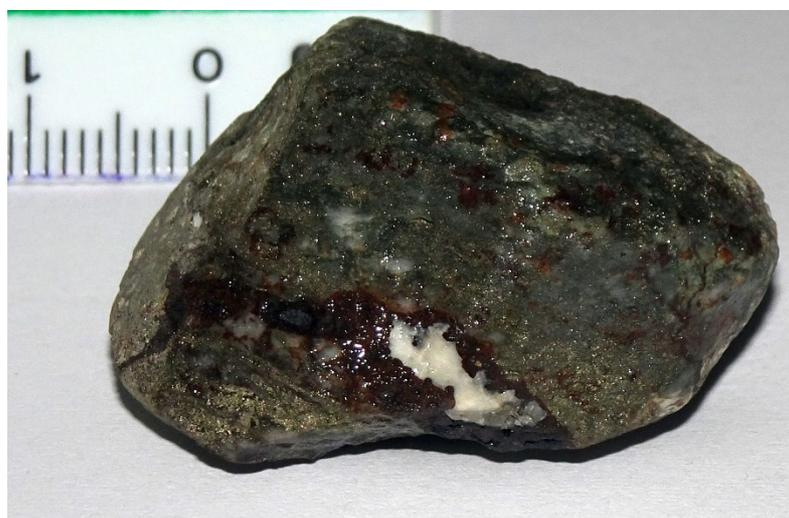
**Figure 3:** Aircore sample from hole JSA20\_175 at 91-92 metres (end of hole) showing phyllic (Quartz-Sericite-Pyrite) alteration and Quartz-Hematite veining with pyritic vein selvage.
