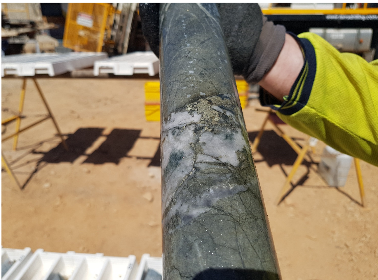
Figure 2. Diamond drill core south of Butchers Creek open pit in hole BCDD372 at 135m below surface shows intense alteration and strongly mineralised veining. Veins comprise quartz, carbonate, pyrite, arsenopyrite and chlorite. Note also the finely disseminated pyrite throughout the altered trachyte host rock
