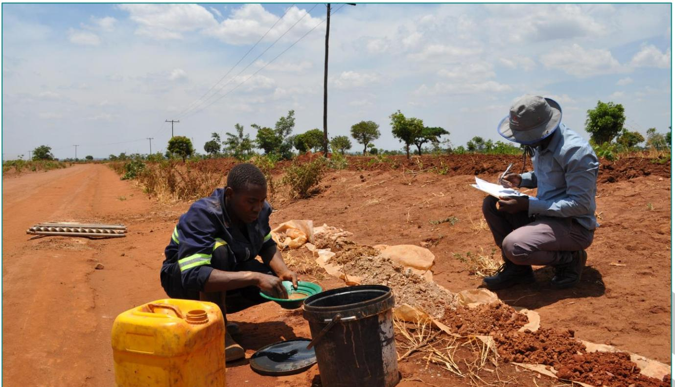
Figure 2. Logging and panning rutile hand-auger samples at Kasiya.
