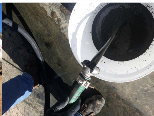
Figure 3: Settled copper concentrate slurry ahead of dewatering
