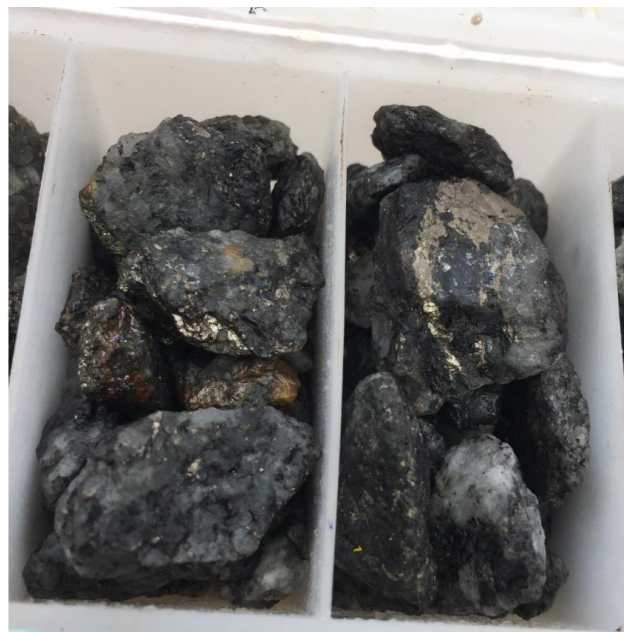
Photo 1. Typical Rebecca pyrrhotite dominant disseminated sulphide mineralisation in RC chip trays Interval is RCLR0572 164-166m (left) ave. 2.43g/t Au, and 166-168 (right) ave. 3.35g/t Au
