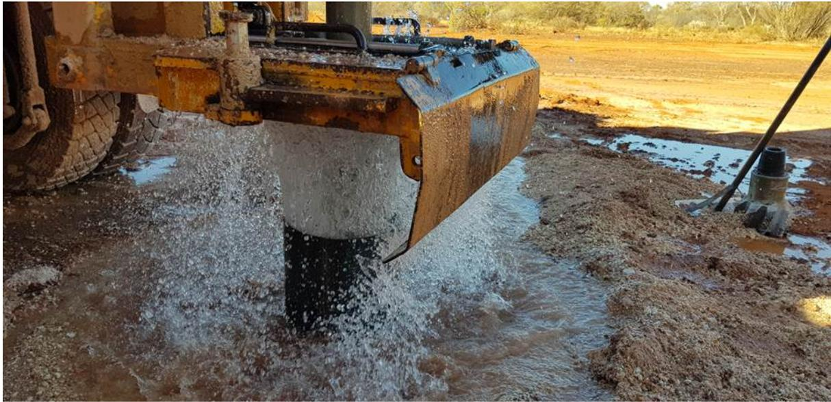
Figure 2: Pump Testing equipment set up to test aquifer yield potential.
