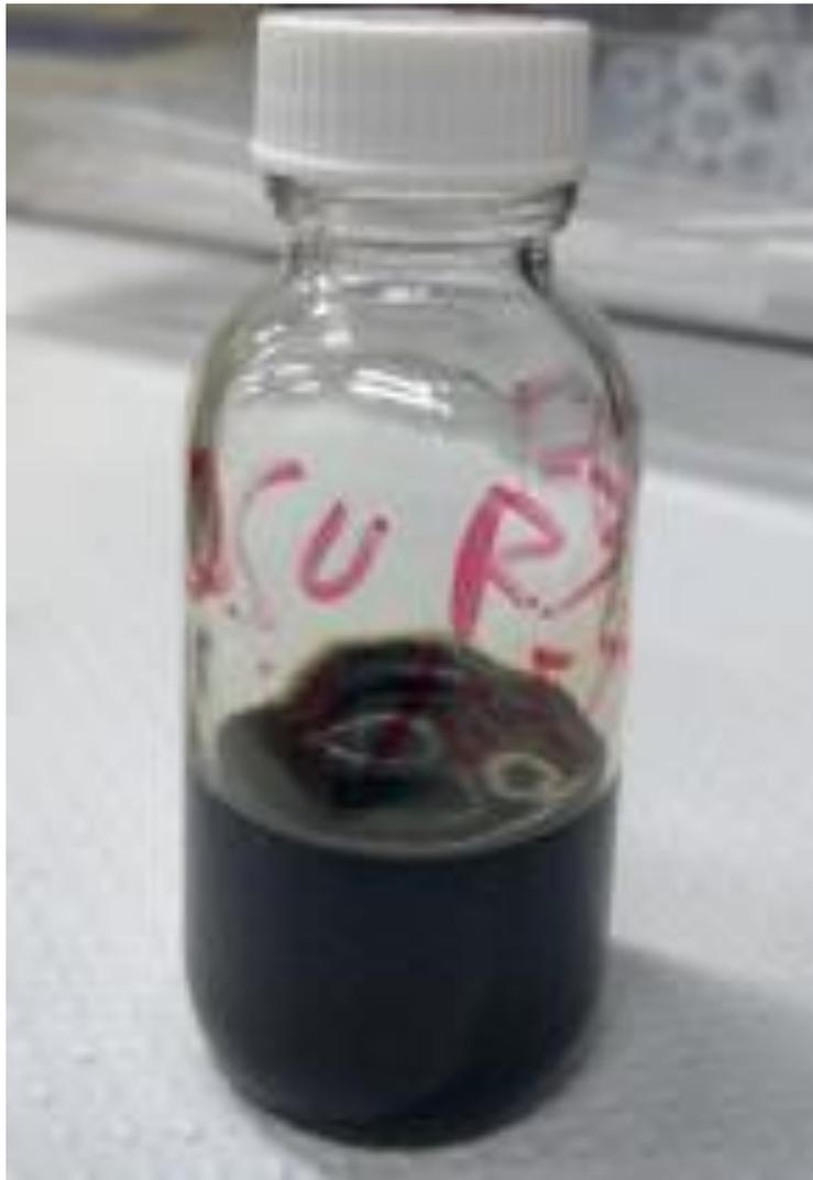
Figure 1: Oil produced from Solvent Extraction of QEM oil shale
