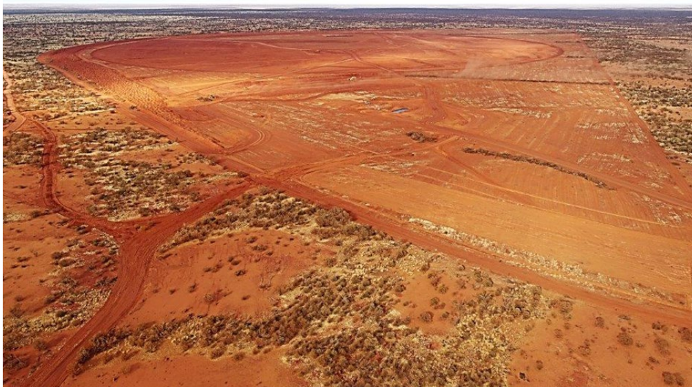
Clearing and topsoil removal for the TSF/IWL
