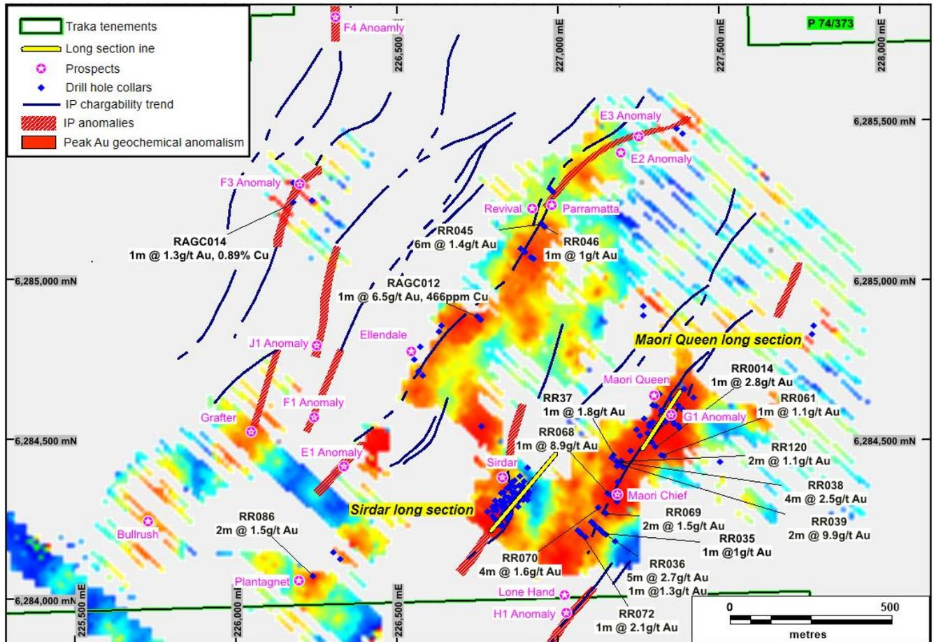
Figure 1. Compilation plan showing existing gold soil geochemical anomalism, IP (Induced Polarisation) survey results, existing prospects and all drill hole collars with selective peak assay results.
